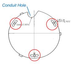
**NOTE:** Depending on the surface where you will install the camera, it may be necessary to drill three (3) holes with  $\phi$  3.5 on the ceiling and use the supplied screw tox.
